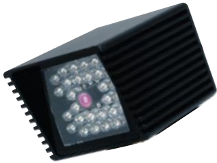
VN571R 30 x IR LEDs · 850nm (20°) - 35M view · 940nm (20°) - 15M view
