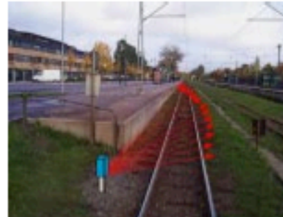
Alarm system for people falling on the rail tracks in a station
