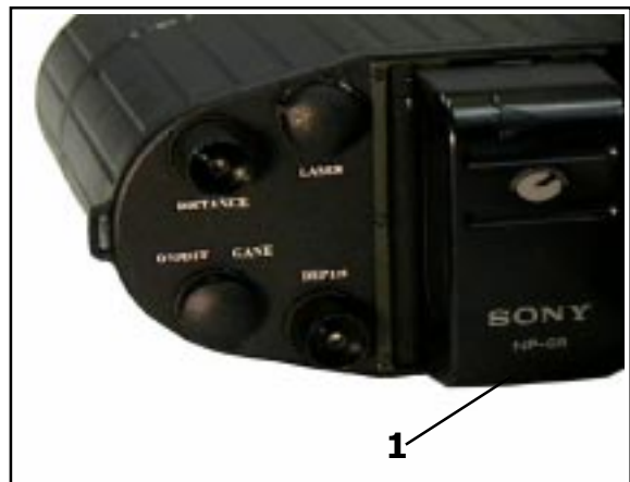
Fig. 4. Control panel with the battery loaded
