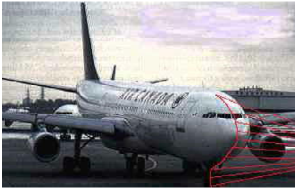
Aircraft radome is tracked by the laser radar system
